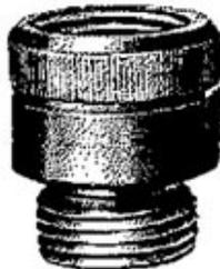
A hose bibb vacuum breaker should be attached to all threaded hose bibbs to which a hose can be connected (unless it has a built-in vacuum breaker), and is required under Article III, Section 42-58, Cross-connection Control and Backflow Prevention.
